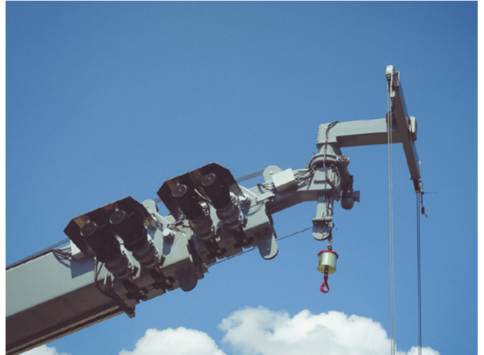
Telescopic jib with spreader bar and auxiliary hoist.
