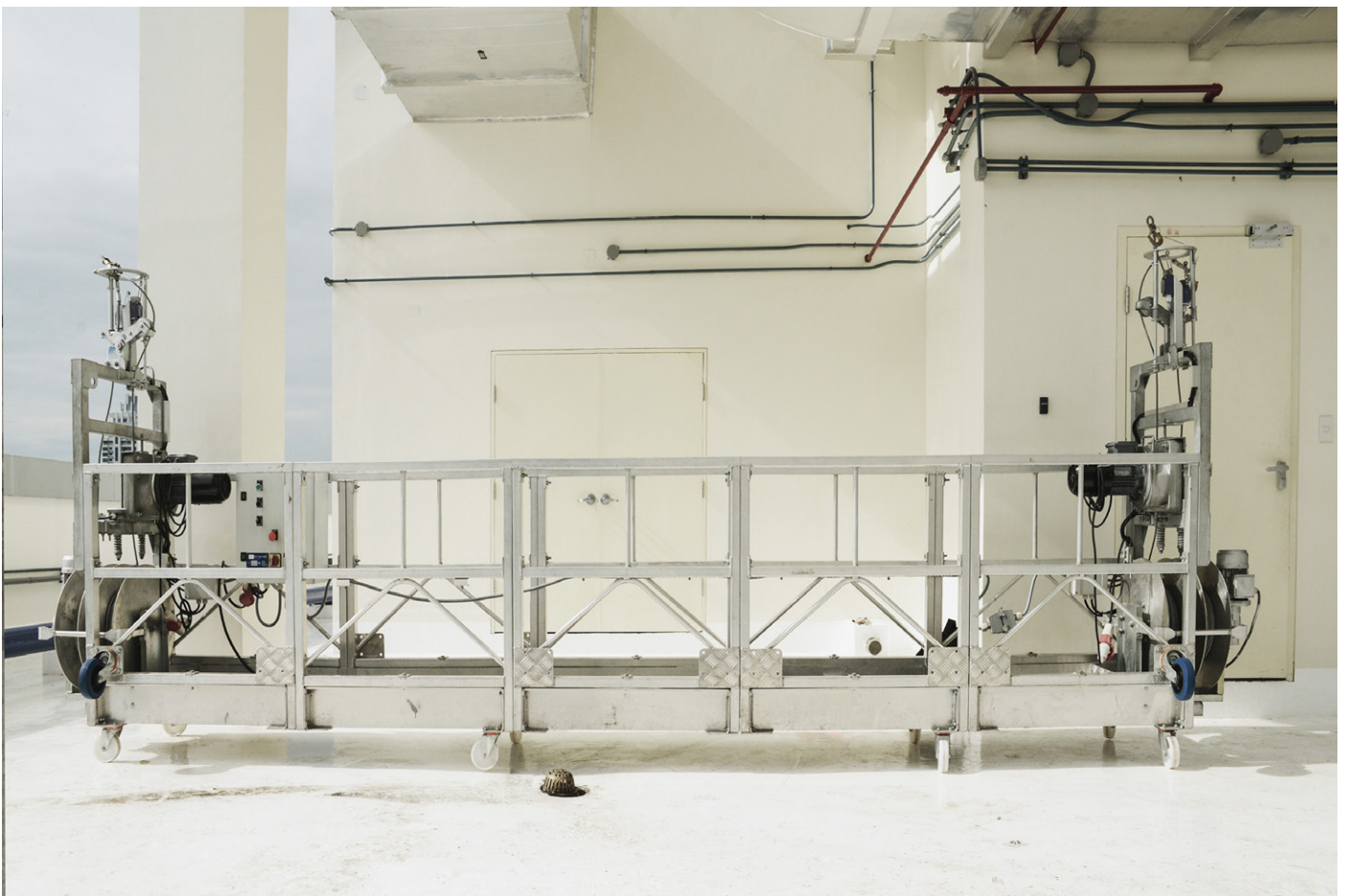
6 meter cradle to be suspended from Davit system.
