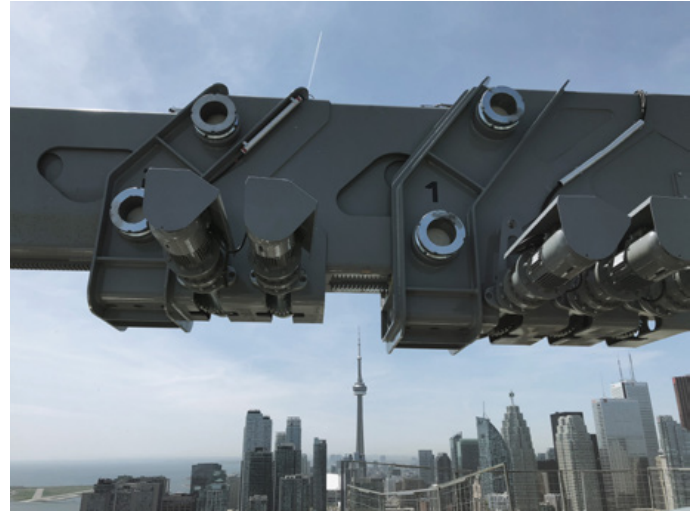
Engines to extend the telescopic arm.
