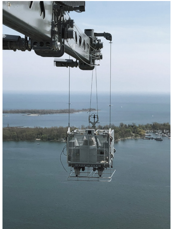
The 3-module suspended cradle towards the Lake Ontario, one of the 5 Great Lakes of North America.
