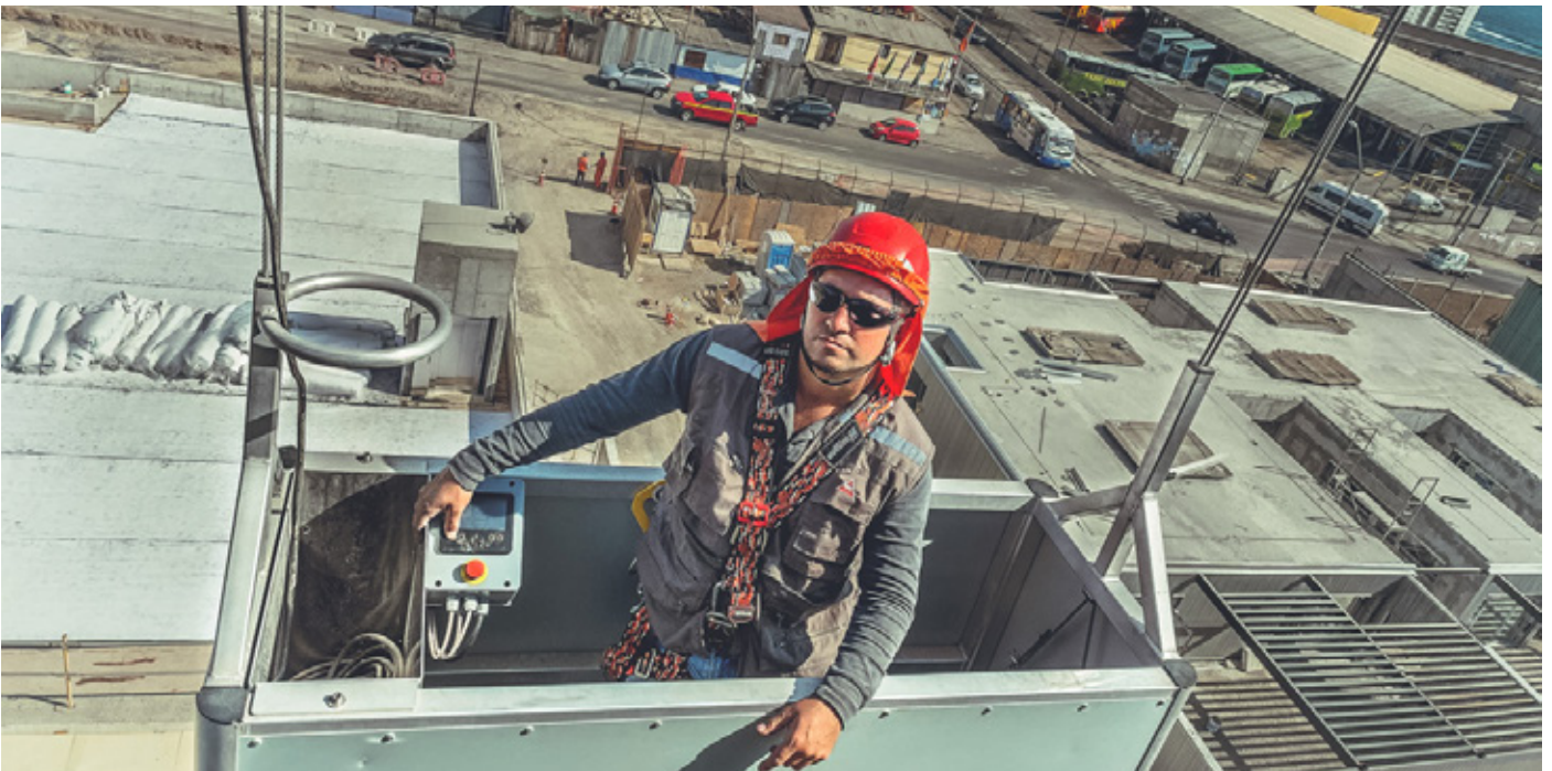
Cradle with control box to operate the translation of the machine and the lifting of the cradle.
