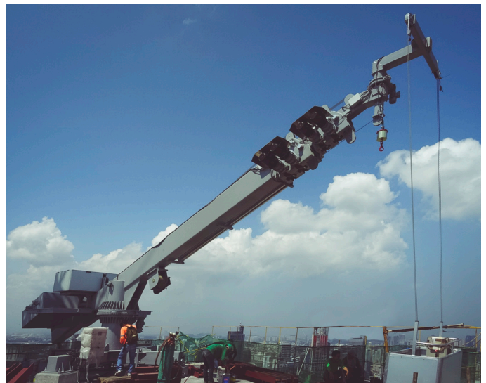
Trump Tower: a compact FBA S machine stationary and through slewing all facades can be reached confortably. Installed in Manila, Philippines.
